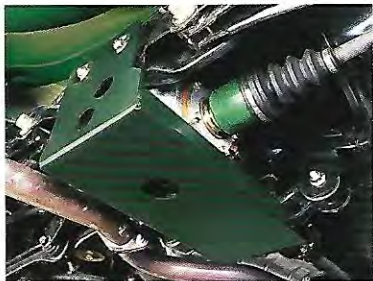
Rear differential protector. Helps protect rear differential from rocks and logs.
