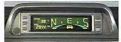
Gauge pack. Displays compass, outside temperature and barometer or altimeter readings.
